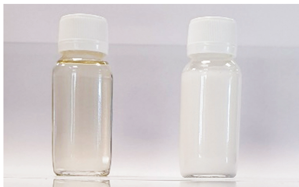
Figure 3. Left: blend of BHT in sunflower. Right: suspension of BHT in water
